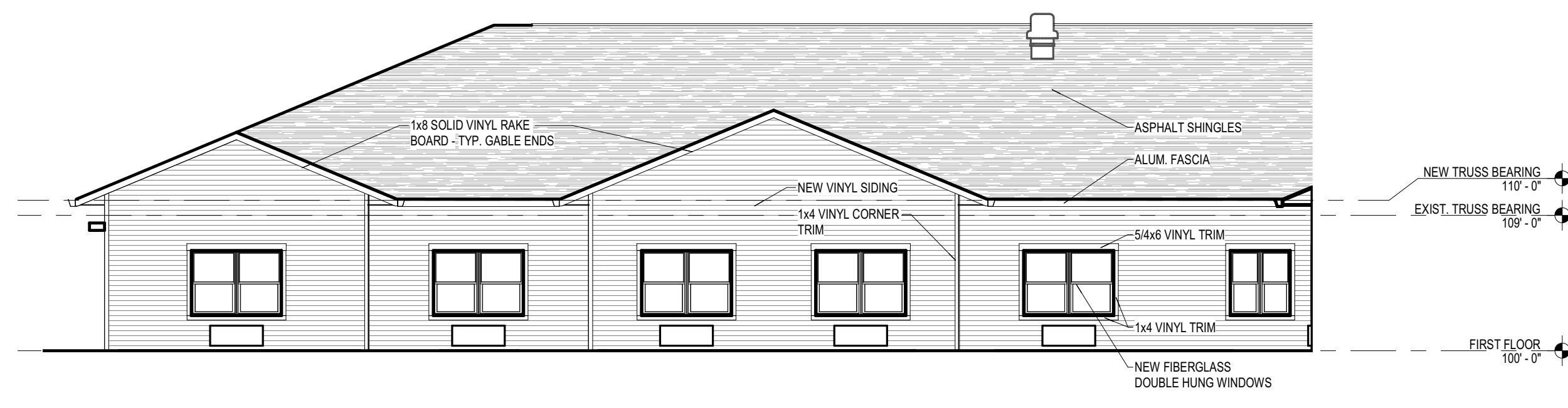
6 UNIT 'D' EAST WING NORTH ELEVATION 1/8" = 1'-0"
